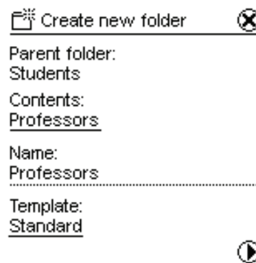
Fig. 5. First step at creating a new subfolder. If the ‘Contains’ checkbox is left unchecked, then we have a grouping folder. The ‘Professors’ link invokes a page allowing the user to select a different database table.
